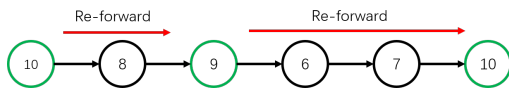
Figure 2: Example of memory cost function for Linear Computation Graph. Number in the vertex denotes its memory cost, and green vertices denotes gradient checkpoints.
