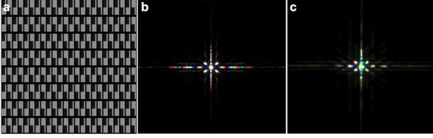
Figure 1. **Comparison of simulated and real-measured PSF.** (a) The pixel layout of a commercial OLED display. Here, different gray-scale values represent different light transmittance of the display. (b) Simulated PSF. (c) Real-measured PSF. The PSFs are brightened to visualize the structured sidelobe patterns.
