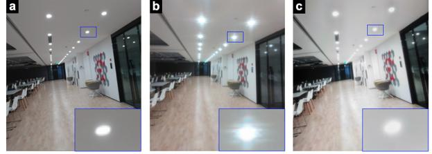
Figure 2. **Comparison of UDC images of real HDR scene and monitor-generated LDR scene.** (a) Real HDR scene captured by a normal camera. (b) Real HDR scene captured by the UDC device. (c) Monitor-generated LDR scene, *i.e.* display the image (a) on a LCD monitor, captured by the UDC device.
