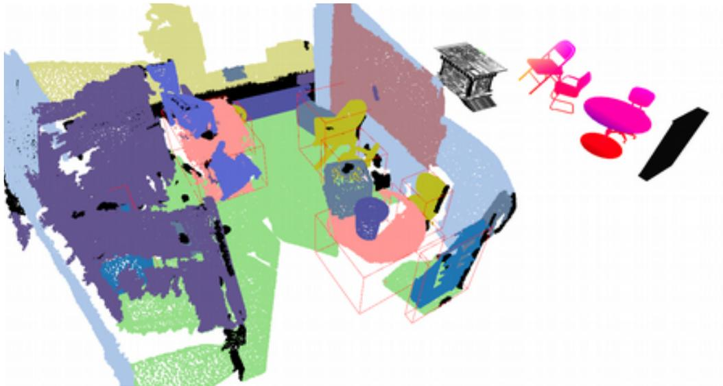
Figure 3: An example synthetic point cloud used for training the network which generates the object proposals. The CAD models corresponding to objects are shown on the right.
