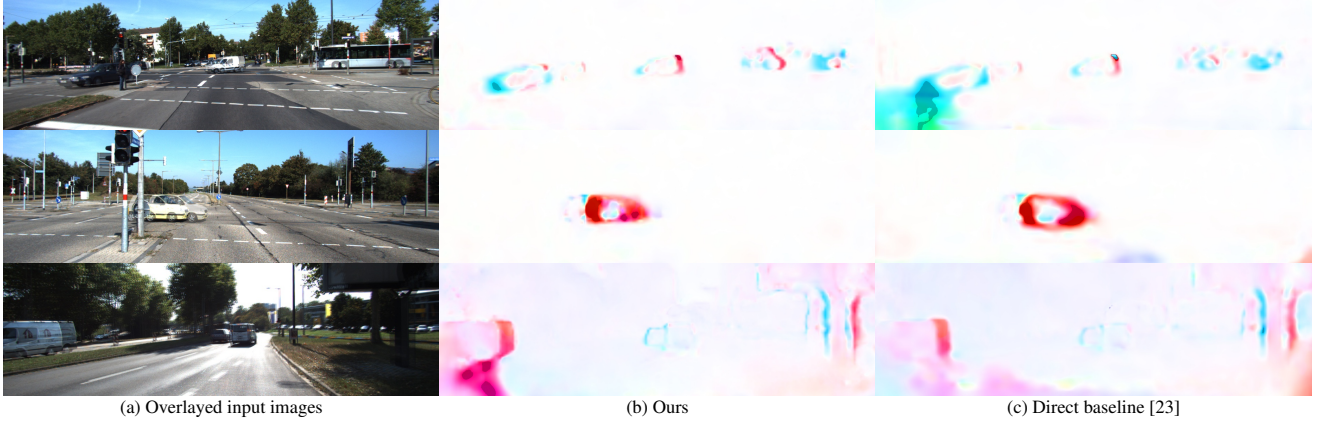
Figure 14. Qualitative comparison of temporal consistency: Each scene shows (a) overlaid input images and scene flow difference maps of (b) our method, and (c) the direct two-frame baseline of [23], visualized using optical flow color coding. Our method provides more temporally consistent estimates near moving objects and out-of-bound regions.
