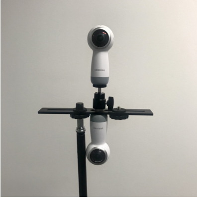
Figure 2. The 360° stereo camera setup we use for capturing the real scene.
