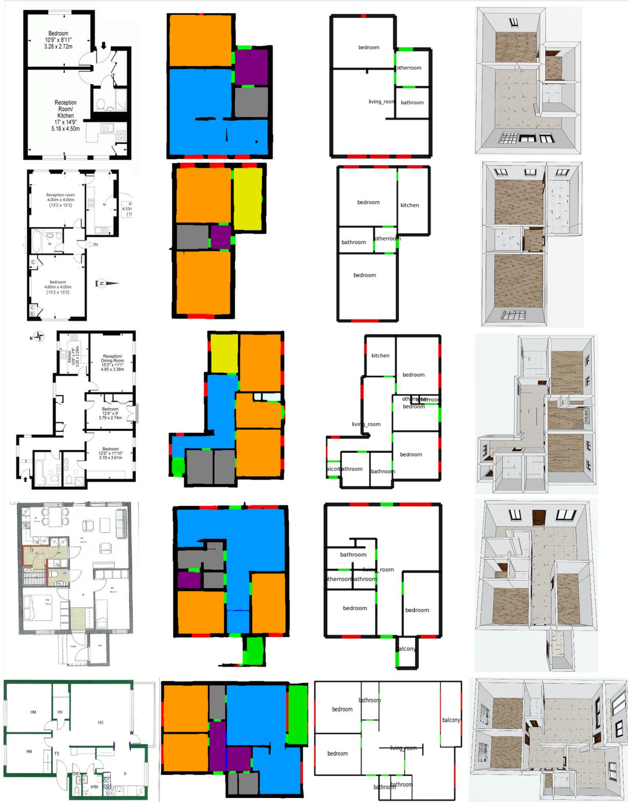
Figure 11. Floor plan recognition and reconstruction results on rent3d(first three rows) and cubicasa5k(last two rows). From left to right, an input floor plan image, semantic segmentation result with post-processing, reconstructed vector-graphics representation with room type annotation, the corresponding 3D reconstruction model.
