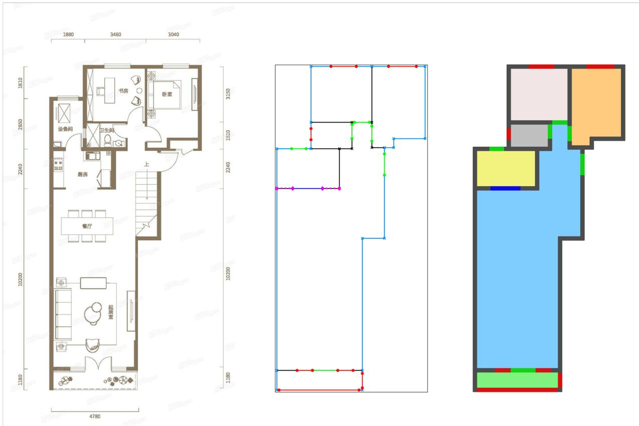
Figure 1. Structural elements annotation. From left to right, an input floor plan image, manual annotation image, rasterized pixel-by-pixel annotation.
