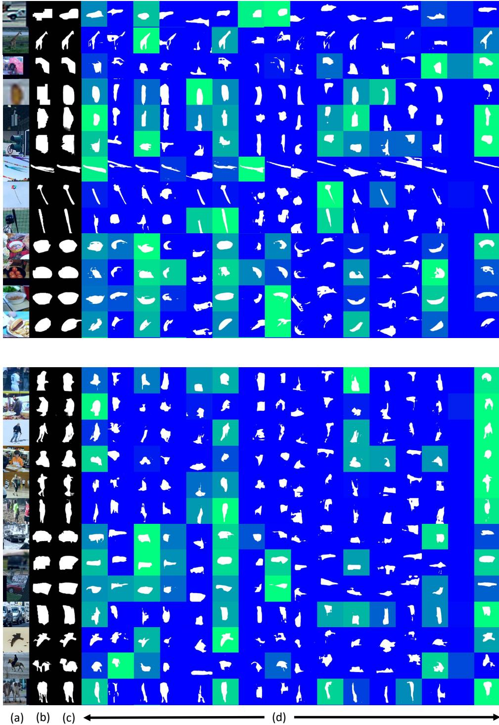
Figure 4. Visualization of 16 latent parts for both training (upper) and test (lower) classes from COCO-20<sup>0</sup> validation set. From left to right: (a) input image, (b) GT segmentation, (c) predicted segmentation, (d) 16 predicted object parts. The predicted importance of the parts is color-coded from blue (smallest) to green (largest).
