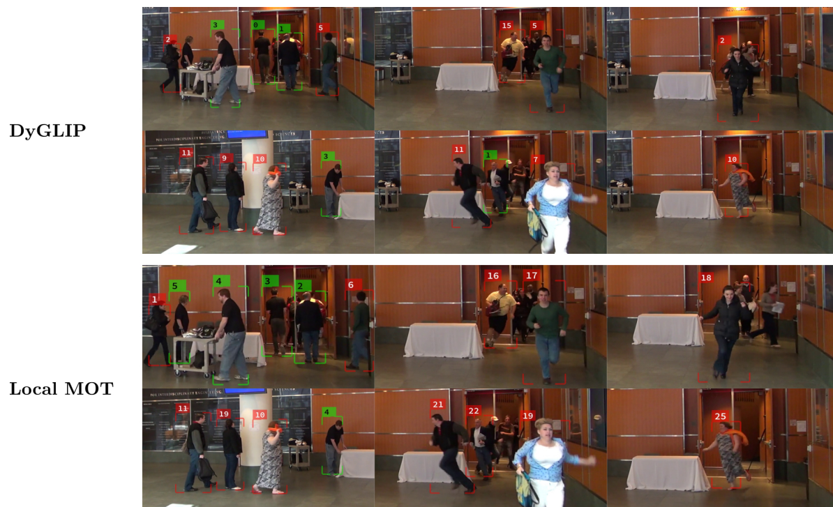
Figure 7. Our proposed method (up) corrects a negative matched case caused by a short-memory MOT system (down). Determined ID is highlighted by the red bounding box.
