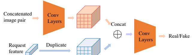
Figure 1. Structure of the discriminator used for adversarial loss.
