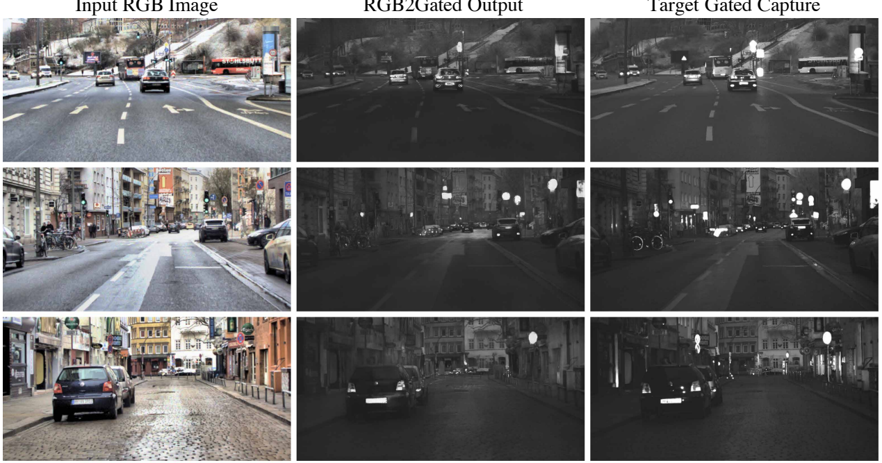
Figure 3: Gated predictions from our RGB2Gated network. Our RGB2Gated network translates tone-mapped clear day RGB captures into gated images. This allows us to train ZeroScatter using experimental gated captures under adverse weather conditions.
