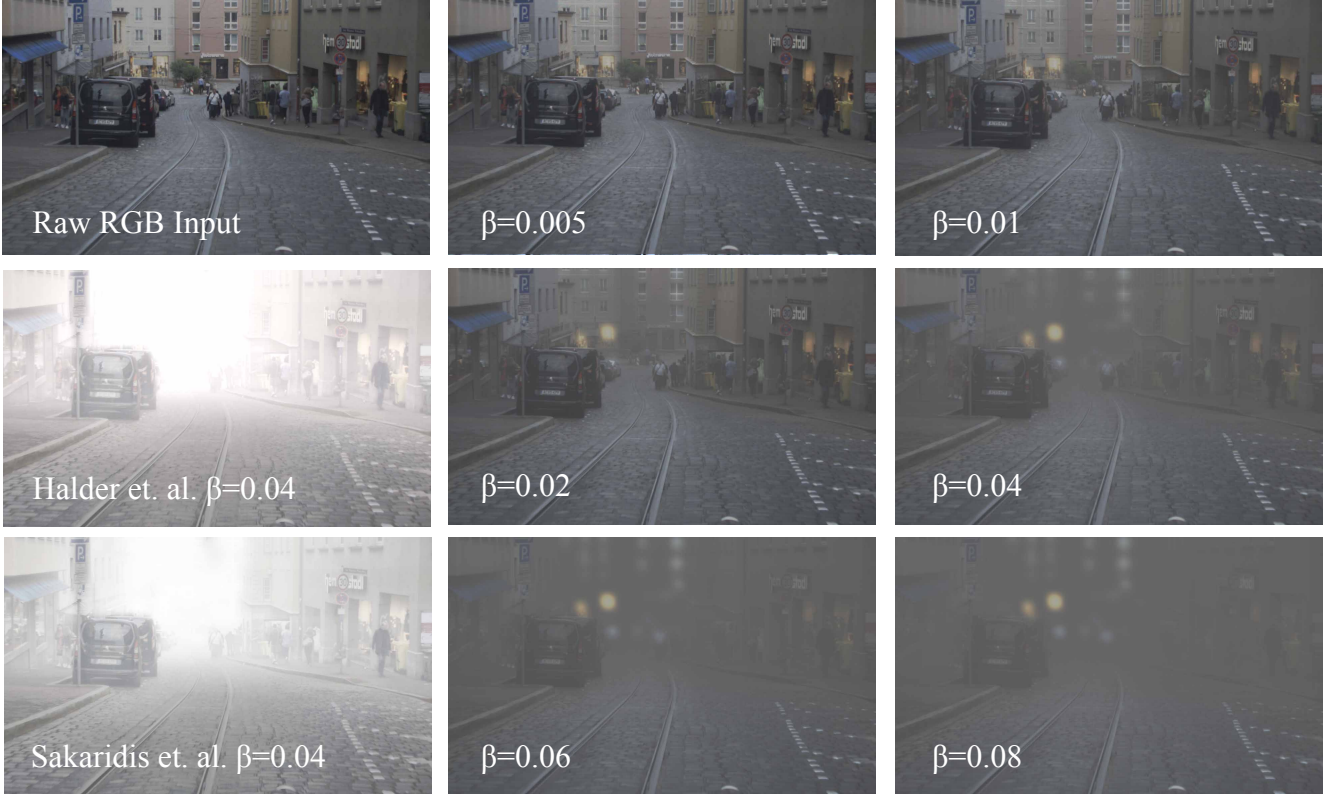
Figure 1: Our adverse weather simulator F_{\text{Syn}} produces a wide range of scattering media. We show qualitative examples for an input clear raw image and increasing fog densities of \beta = 0.005, 0.01, 0.02, 0.04, 0.06, 0.08 . We also show a comparison to Halder et al. [16] and Sakaridis et al. [29] at fog density \beta = 0.04 . These methods over-estimate airlights and produce unrealistically bright scatter.
