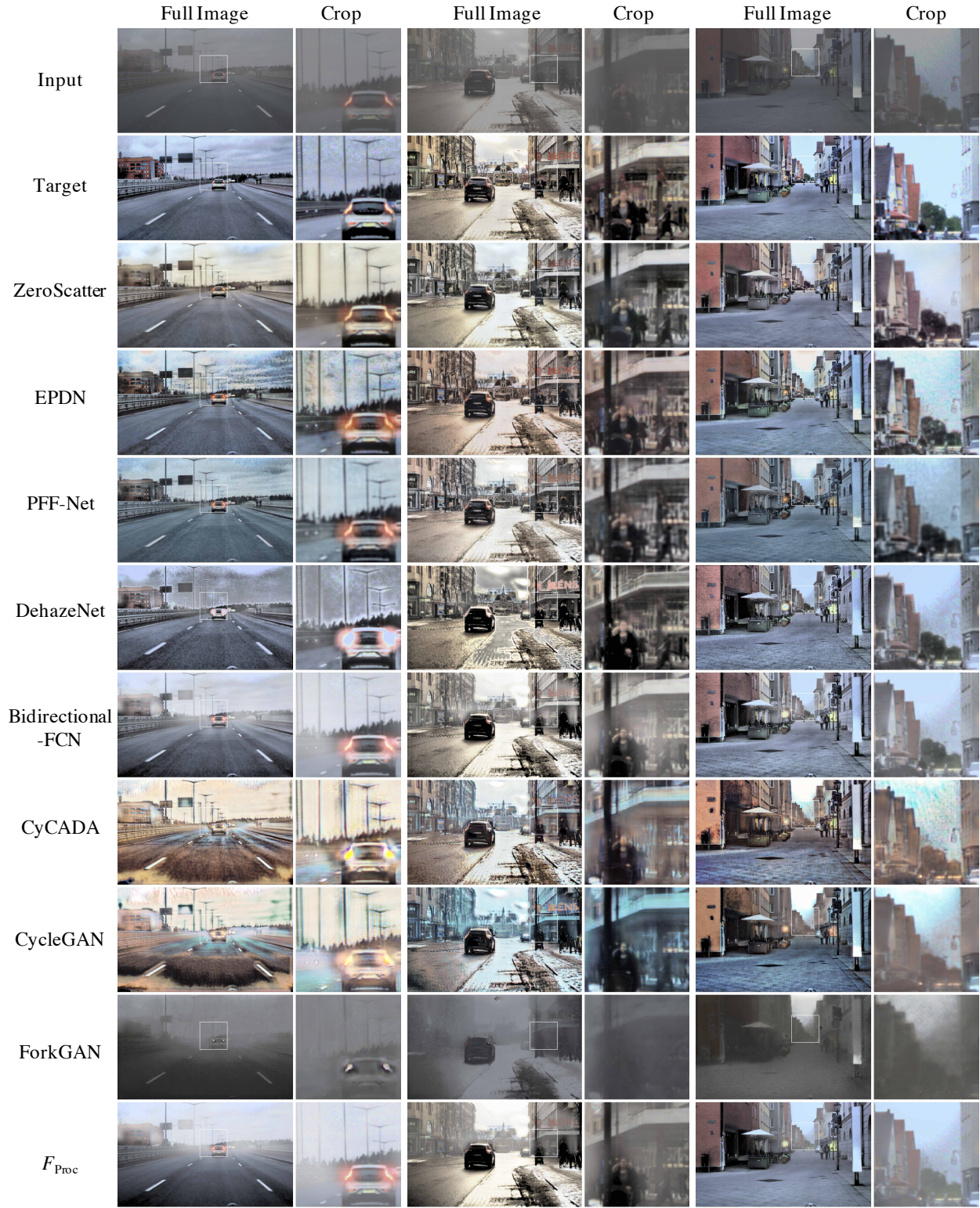
Figure 8: Qualitative performance comparison on scenes with synthetic adverse weather. Compared to the baseline methods, ZeroScatter is less affected by the halos around lights, which can be seen in the first example. ZeroScatter produces accurate, high contrast outputs without amplifying noise, as shown in all three examples.
