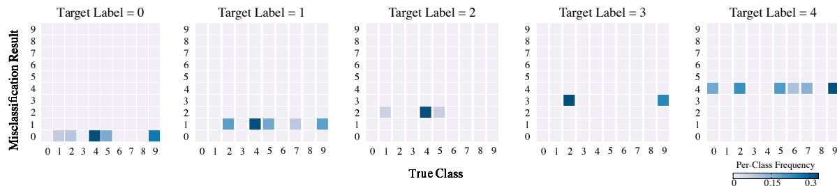
Figure 16: Heat plot on the classification outcome when a clean data is misclassified by the backdoored model. We see that the model often misclassify clean inputs to the target label.
