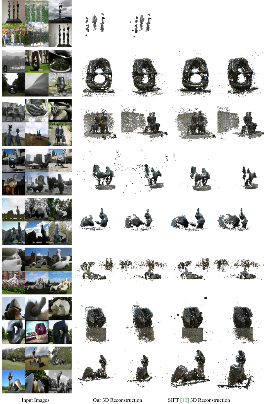
Figure 10: Additional SfM results. Randomly selected input images and 3D models reconstructed using our matches and those obtained using the SIFT [10] baseline. This figure demonstrates the variety of the input images and their scene shift as well as that both our and [10] are of similar quality for these image sets. However, unlike [10], our model is able to determine that there are 3 statues in the first example.
