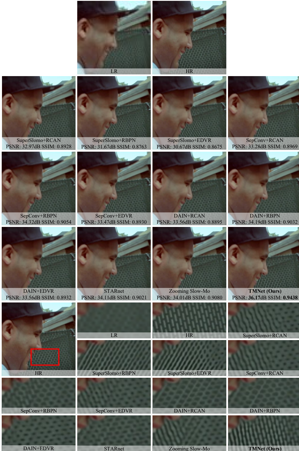
Figure 7: Quantitative and qualitative results of our TMNet and other STVSR methods on Clip 0723 of “00085” in Vimeo-Medium [12]. For two-stage STVSR methods, we employ SuperSloMo [5], SepConv [7] or DAIN [1] for VFI and RCAN [13], RBP [2] or EDVR [9] for VSR. For one-stage STVSR methods, we compare our TMNet with STARnet [3] and Zooming Slow-Mo [11]). The best results on PSNR (dB) and SSIM [10] are highlighted in bold .
