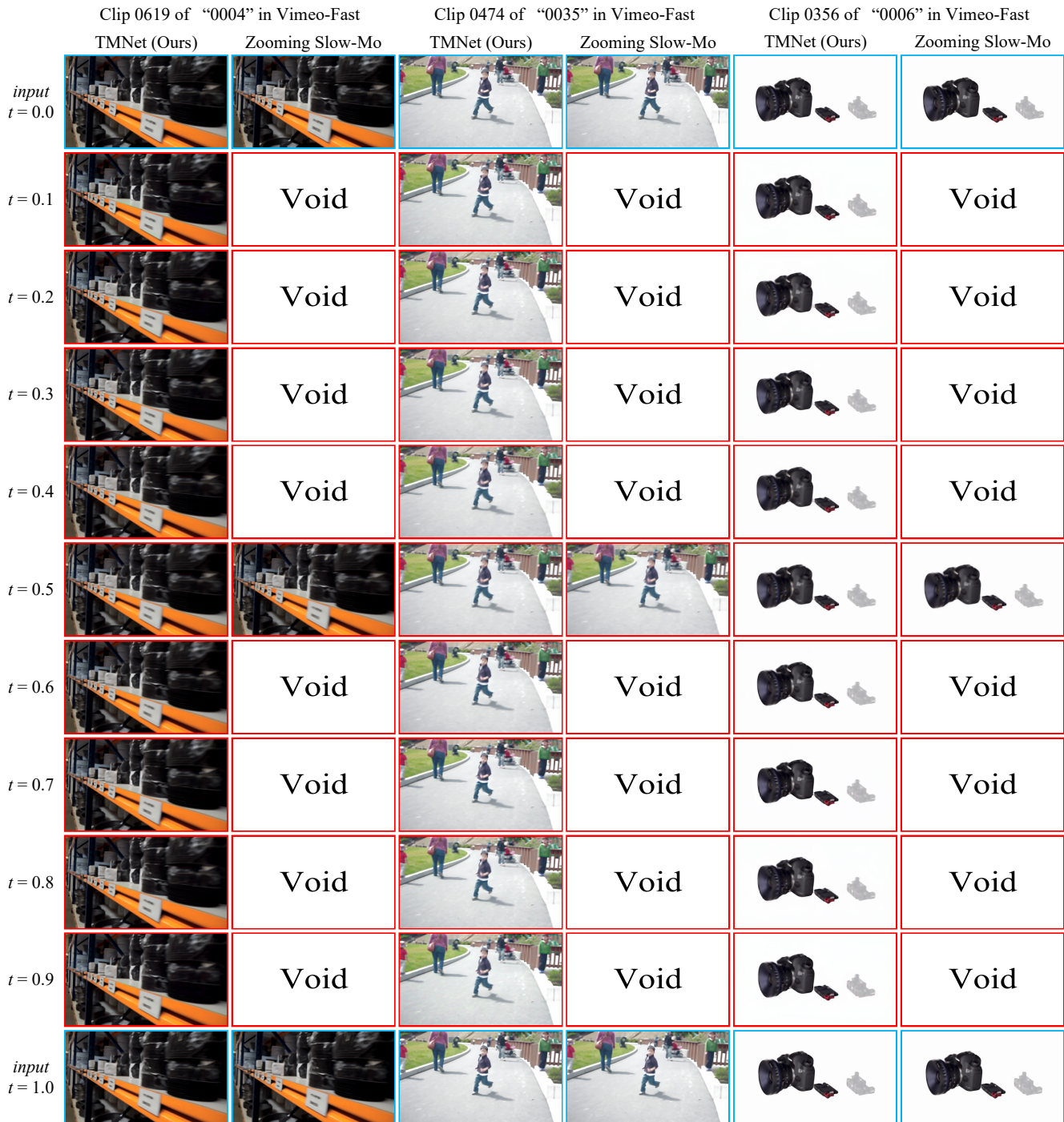
Figure 3: Comparison of flexibility on STVSR by our TMNet (1-st, 3-rd, and 5-th columns) and Zooming Slow-Mo [11] (2-nd, 4-th, and 6-th columns) on three video clips from the Vimeo-Fast dataset [12]. We show the intermediate frames between the adjacent two frames according to the temporal hyper-parameter t \in \{0.1, 0.2, 0.3, 0.4, 0.5, 0.6, 0.7, 0.8, 0.9\}
