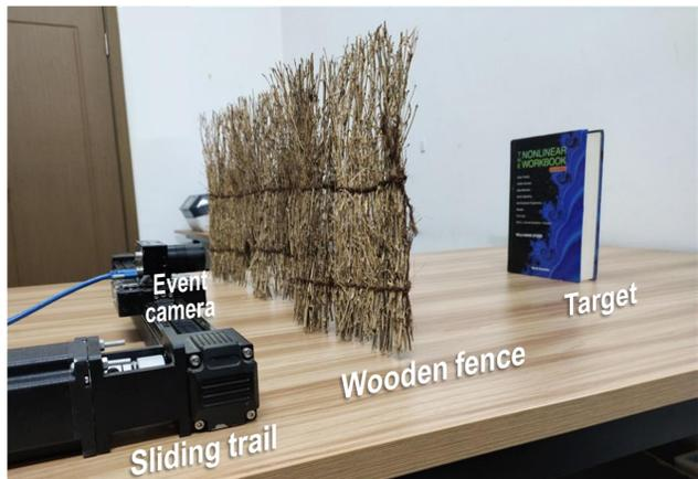
Figure 1: An example of our experimental scenes. It consists of occlusions (wooden fence), targets (book) and an event camera installed on a programmable sliding trail.
