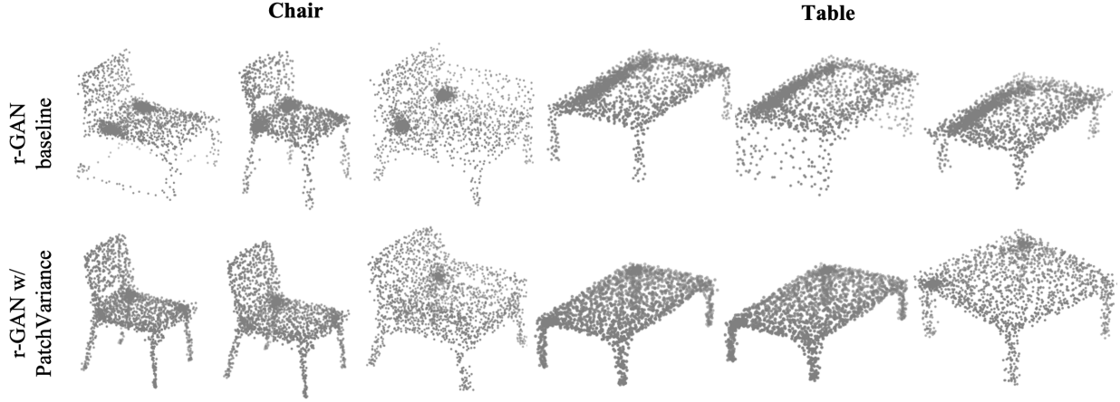
Figure 1. Validation of the significance of PatchVariance on r-GAN [1]. Non-uniformity issue is a common problem faced by point cloud GANs, our PatchVariance loss directly works on the generated point cloud, and is invariant to the architecture of the generator, hence it effectively enhances the uniformity of generated point clouds for r-GAN as well. Darker regions have a higher density of points
