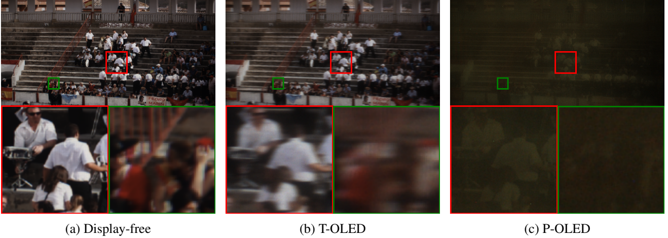
Figure 1: More real data samples acquired by our MCIS set-up. (a) The image captured with camera covered by thin glass, (b) T-OLED, and (c) P-OLED.
