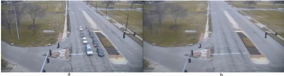
Figure 4a. left - Background image using median frames over 30 seconds, right- Background image using median frames over 180 seconds
