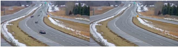
Figure 4b. left - Background image for a pixelated video using median frames over 30 seconds, right - Background image using median frames over 180 seconds
