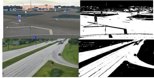
Figure 6. Road mask generation for filtering out false anomaly candidates.
