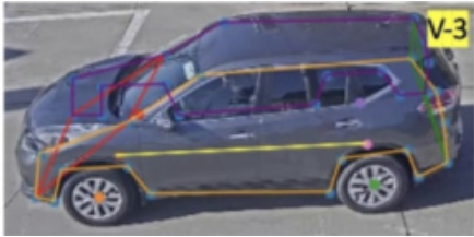
Figure 2. Example of vehicle keypoint detection and surfaces and direction estimation. [11].
