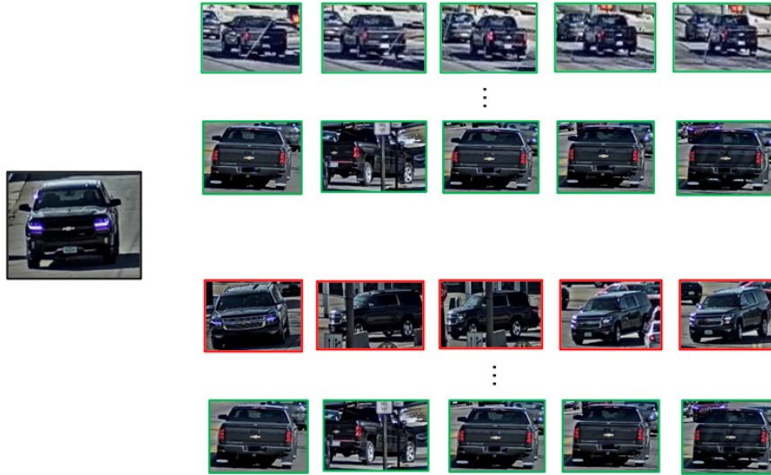
Figure 3. Example of the visual results for the proposed ReID system. The image on the left is the query while the images on the right are the candidates. The lower rows are the results obtained with the baseline. Then, the upper rows are the results of applying the proposed enhancements. Green boxes represent true positives and red boxes false positives.
