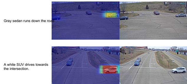
Figure 1. Examples of proposed SBNet output. With natural language and an image, it finds the corresponding area in the image and shows high activation in that area. The left column is the natural language description, the center column is the model’s output activation mask, and the right column is the input image.
