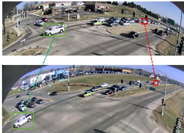
Figure 6: Vehicles with similar appearance are matched in the order in which they appear in the camera.
