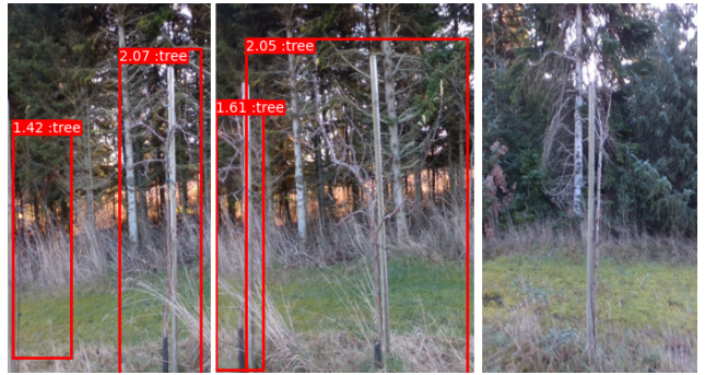
(b) The three images show false positives, badly sized bounding box, and false negative, respectively
