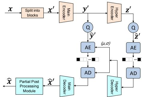
Figure 1: General Framework Illustration of Variational Autoencoder (VAE)-based Image Coding
