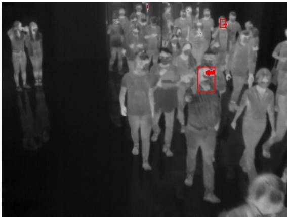
Figure 9. Thermal image of a crowd walking past our system where two subjects at different sensor-subject distances have simulated elevated forehead temperature. After thermal compensation, our system successfully identified the two subjects (red boxes) in real-time using a single alarm threshold.
