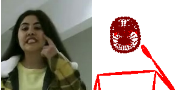
Figure 5. Example of hand-face interaction, where the pose estimation fails for the interacting hand (Holistic).
