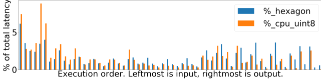
Figure 2: Per layer profiling of MobileNetV3 minimalistic on Pixel4 CPU uint8 and DSP (Hexagon). The leftmost is the input layer while the output layer is on the right.
