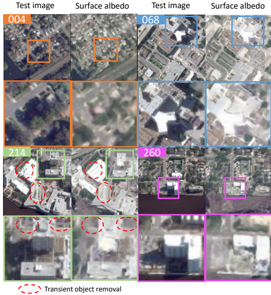
Figure 6. Demonstration of S-NeRF shadow removal and transient object removal. The first and third column show unseen test images and the second and last column show the estimated albedo at the surface. The approach is mostly successful in restoring color to the persistent shadows. Remaining errors are particularly found at the intersection between the ground and vertical facades and along their outer edges. We can also note the transient object removal in the three parking lots circled in area 214 (lower left).
