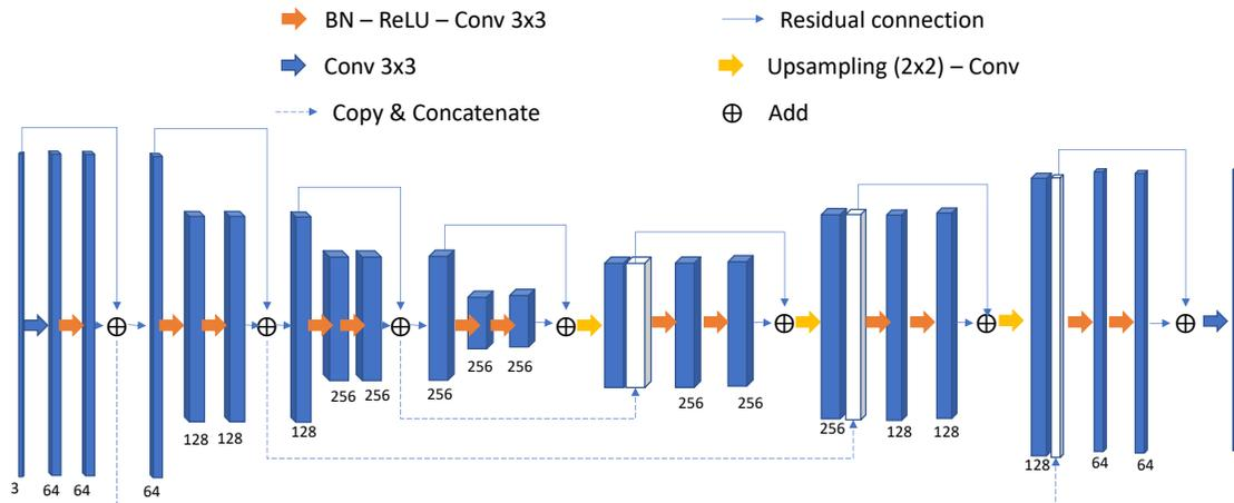
Figure 2. Residual U-Net architecture used for vegetation segmentation
