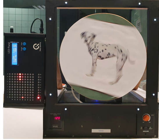
Figure 3. Our experimental setup. The eight white LEDs are coplanar with a controlled spinning wheel for spatial alignment of cameras. The LED panel (on left) is used for temporal synchronization.
