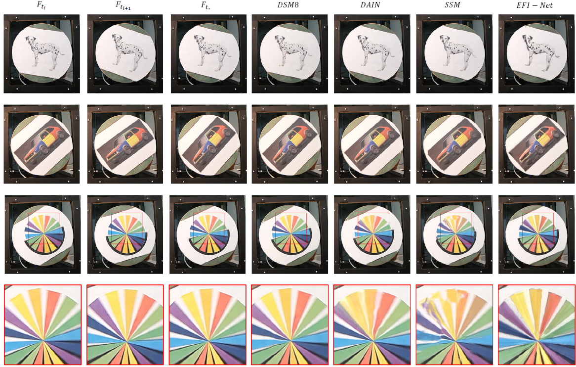
Figure 7. Interpolated frames of EFI-Net, SSM [22], DSM8 [45], and DAIN [2] on our dataset. The sequences from top are: car 100 RPM, dog 100 RPM, star 150 RPM. Bottom row is zoomed in on star 150 RPM, highlighting the artifacts of the different methods.
