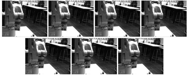
Figure 8. Entire sequence of 7 frames from the left camera for angle estimation.
