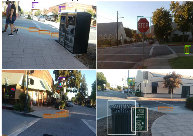
Figure 7: Object detection model detecting traffic signs, traffic lights, road signs, trash can and yellow pavement.
