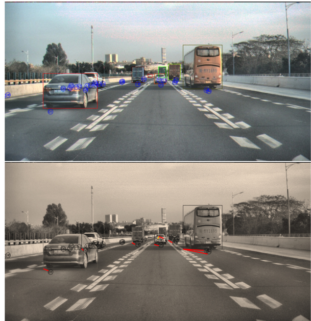
Figure 1: An illustration of the associations between radar detections (radar pins) and camera detections (2D bounding boxes). The context of the scene is illustrated in the top picture, with the image captured by the camera along with the detected bounding boxes and the projected radar pins (shown as numbered blue circles). The bottom picture adds red lines to highlight the association relationships between radar pins and bounding boxes. The tiny orange line in the middle denotes uncertain association relationship, which will be explained later.
