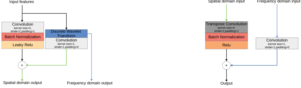
Figure 3: Left:DWT down-sampling module. Right:DWT up-sampling module.
