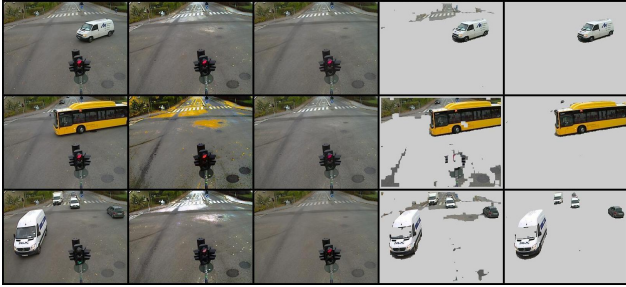
Figure 4. Example images for background foreground segmentation. Left: Input images. Second column: Transformed background image using [9]. Third column: The same using proposed method. Fourth and fifth columns: Segmented output based on the two methods. See also supplemental material.
