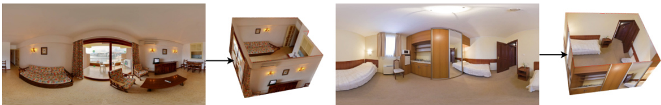
Figure 1. Illustration: Our OmniLayout can predict both non-cuboid layout as well as cuboid layout from the input RGB panorama.
