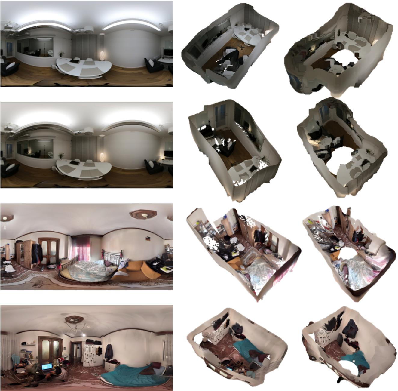
Figure 11: Qualitative results using in-the-wild data. On the left the input color panoramas are depicted. The two top rows are captured with a 360° camera, while the bottom two rows are stitched panoramas from a mobile phone. The colored point clouds of the predicted depths from our UNet model (middle) and BiFuse [8] (right). Ceilings have been removed for visualization purposes.
