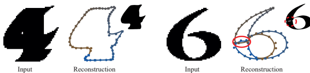
Figure 11: Limitations. Im2Vec is only supervised by an image-space loss, so it can sometimes miss small topological features (Left), or produce semantically meaningless or degenerate geometries (Right). While the former can be resolved by providing higher resolution supervision, the later could be mitigated by using local geometric priors.
