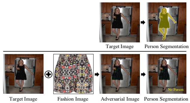
Figure 1. Overview of our proposed Fashion-Guided Adversarial Attack (FashionAdv). Top row: person is segmented successfully. Bottom row: given a target image and a guided-fashion style image, FashionAdv synthesizes natural clothing texture that can nevertheless fool a person segmentation network by making the person invisible to the network.
