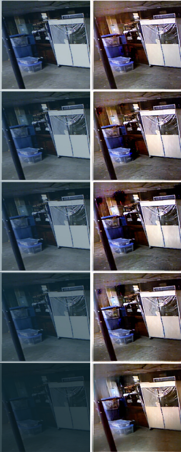
Figure 6. Synthetic underwater image rendered using NYU Depth data set considering Equation 7 and corresponding restored images. First column shows rendered underwater images for ocean water (Type I, IA, IB, II, III) as per Jerlov [10]. Second column shows corresponding restored underwater images using proposed pipeline.
