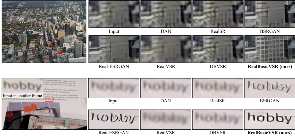
Figure 11. Qualitative Comparison. Our RealBasicVSR is able to aggregate long-term information effectively. It generates much more details when compared to existing works. In particular, by aggregating long-term information through propagation, RealBasicVSR successfully restores the word “hobby”, which can be clearly seen in latter frames. (Zoom-in for best view)
