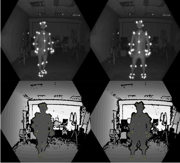
Figure 3. Two examples of marker detection results using the K4A sensor. On the top row, the IR images are depicted where the retro-reflective markers are clearly identified. On the bottom row, the IR detections (green stars) are overlaid on top of the depth maps, inside the empty/invalid depth measurement regions that correspond to the retro-reflective "blind" spots for the K4A sensor.
