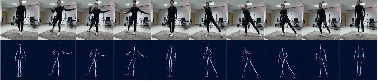
Figure 6. A representative example of a captured motion sequence: (top) the physical scene and the actress as perceived by an observer; (bottom) the real-time output of our system rendered as 3D skeleton along with markers frames.
