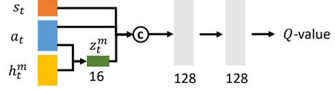
Figure 2. The architecture of the  $m^{th}$  agent in the team. Note that each agent shares the similar model architecture but with its own parameters.  $a_t$  and  $h_t^m$  are first fed into a linear layer with ReLU activation to generate feature  $z_t^m \in \mathbb{R}^{16}$ .  $z_t^m$ ,  $a_t$  and  $s_t$  are then concatenated and passed through three linear layers with ReLU activation in between to output the  $Q$ -value.
