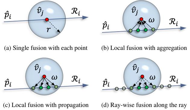
Figure 4. Toy examples of different fusion methods. The red point  $\hat{v}_j$  denotes the anchor voxel with LiDAR points. Green points in  $\mathcal{R}_i$  indicate voxel bins  $v_j$  within the ball with radius  $r$ . The dotted line in 4d represents the assigned existence probability for training.
