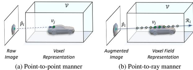
Figure 1. Compared with previous work [17, 50] in **1a** that projects feature from raw image to voxel and represents in a *point-to-point* manner, the proposed method in **1b** projects feature from augmented image to voxel field and represents in a *point-to-ray* manner. Dotted and solid arrow denote point- and ray-level projection.
