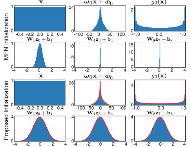
Figure 3. Comparison of distribution of activations at initialization. The initialization scheme proposed for MFNs [17] results in vanishingly small activations for deep networks (shown for layers 0, 1, 4, and 8). The proposed initialization scheme maintains a standard normal distribution after each linear layer (all distributions shown for a network with  $d_h = 1024$ ), and activations at intermediate outputs closely match our analytical derivations (red lines, see supplemental for details).
