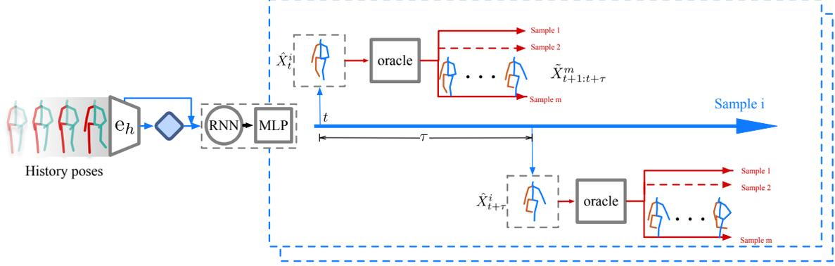
Figure 3. The procedure of short-term oracle supervision. During training, we can get several predicted human motions. For each sample (indicated by the blue arrow), the poses will be fed to the oracle after each  $\tau$  time steps. The oracle will provide several possible future poses as options. The predicted human motions only need to be similar to one of the options in each short time horizon.
