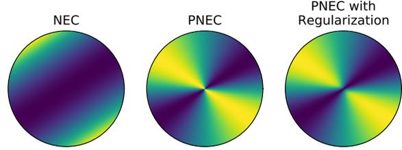
Figure 4. Visualization of the NEC, the PNEC, and the PNEC with the regularization proposed in Sec. 4.5. The plot shows  $\mathbf{t}$  in a neighborhood of  $\mathbf{f}$  (in polar coordinates), where the center of the circle corresponds to  $\mathbf{t} = \mathbf{f}$ . For  $\mathbf{t} = \mathbf{f}$ , the PNEC shows a finite discontinuity, for which the limit depends on the direction. Our regularization eliminates this singularity while also maintaining the overall shape of the energy function.
