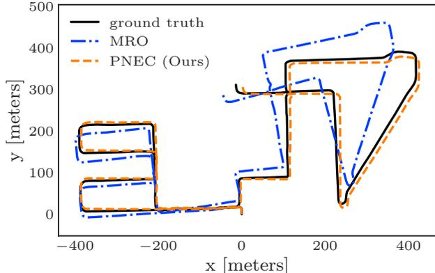
Figure 7. Qualitative trajectory comparison for KITTI seq. 08. The trajectory was generated with the estimated rotations of MRO [9] and PNEC, respectively, and are combined with the ground truth translations for visualization purposes. Relative rotations computed with the proposed PNEC lead to a significantly reduced drift.
