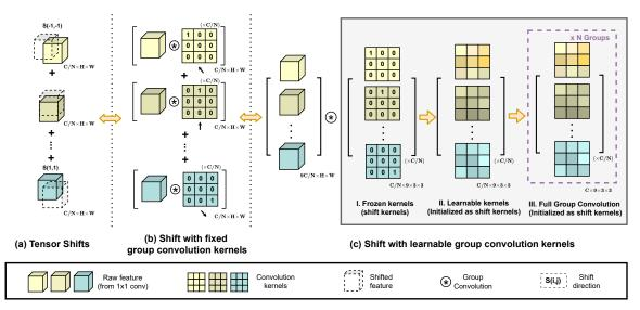
Figure 3. Practical improvements on shift operations. (a) Simple implementation with tensor shifts. (b) Fast implementation with carefully designed group convolution kernels. (c) Further adaptations with learnable kernels and multiple convolution groups.
