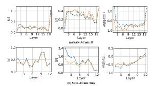
Figure 5.  $|\alpha|$ ,  $|\beta|$  and  $log(|\alpha/\beta|)$  from different layers of SAN-ACmix and Swin-ACmix. Lines in the same plot correspond to parallel experiments. The final output is computed as  $F_{\rm out}=\alpha \cdot F_{\rm att}+\beta \cdot F_{\rm conv}$ .
