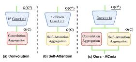
Figure 1. A sketch of ACmix. We explore a closer relationship between convolution and self-attention in the sense of sharing the same computation overhead ( $1 \times 1$  convolutions), and combining with the remaining lightweight aggregation operations. We show the computation complexity of each block *w.r.t* the feature channel.
