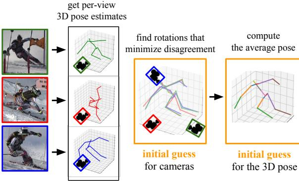
Figure 4. **Initialization** – We form an initial guess for the 3D pose and the cameras by taking the mean of rigid aligned 3D poses estimated from each RGB image using an external single-view weakly-supervised 3D pose estimation network [37, 62].
