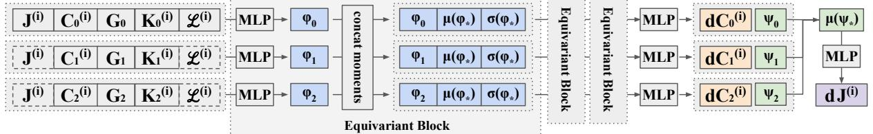
Figure 6. **Architecture** – In order for predicted updates to respect symmetries of the problem at hand, we copy and concatenate view-invariant inputs (current pose estimate, average heatmap likelihood - dashed line) to each row of view-specific inputs (current cameras and joint projections, heatmaps), pass them through a Permutation-Equivariant MLP Block shown above. To get permutation-invariant final pose update we additionally apply MLP to averaged output pose embeddings.
