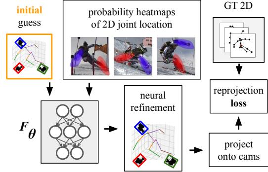
Figure 5. **Refinement** – We train a *neural optimizer*  $f_\theta$  to predict iterative refinement that minimizes the reprojection error with the ground truth re-projection, using the current guess and joint heatmaps as an input. During inference, we *do not* need ground truth 2D projections.
