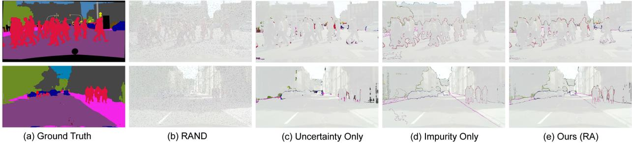
Figure 4. **Visualization of queried regions to annotate (2.2%) on GTAV → Cityscapes.** Compared to simple RAND baseline, Uncertainty Only, and Impurity Only, Ours (RA) is able to select the most diverse and uncertain regions of an image. Please zoom in to see the details.
