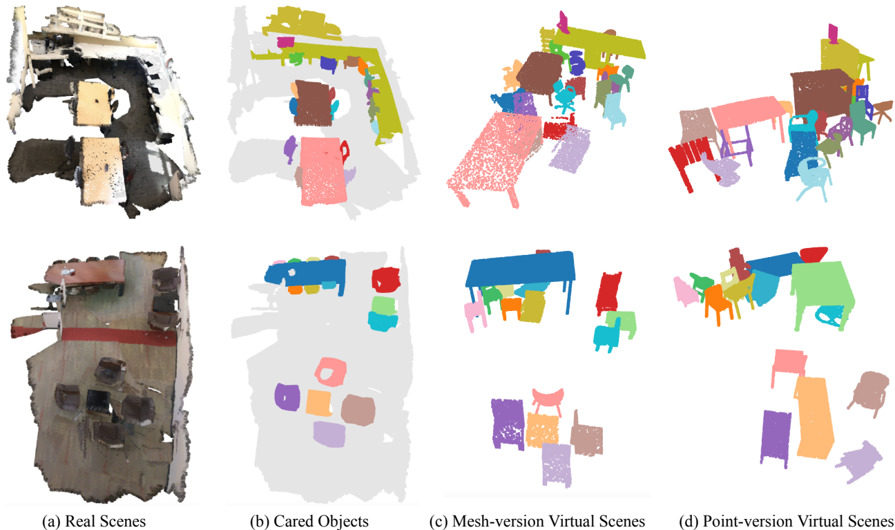
Figure 5. The qualitative visualization results of our virtual scene generation. In (b), (c) and (d), the same color indicates the same object. Gray points are floors, walls and objects that we do not care. It can be seen that the virtual scenes preserve the coarse scene context and the supporting relationships between objects.
