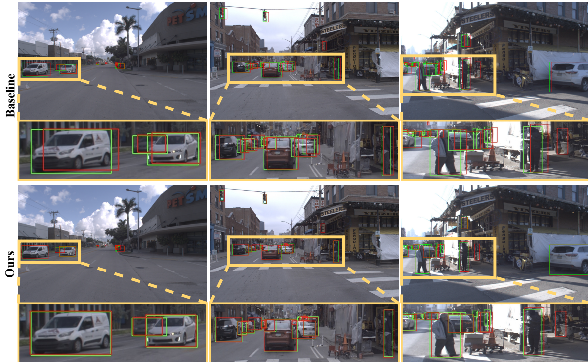
Figure 6. Visualization results of the baseline detector and the proposed method. The green boxes represent ground truth boxes, while red ones represent prediction results.
